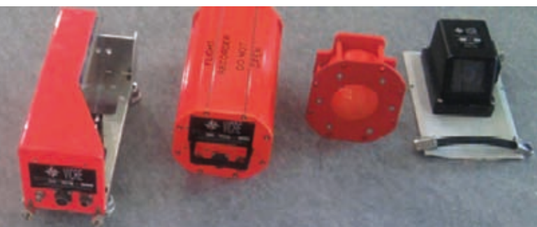
VICRE system with Flight Recorder, Crash Memory, and one Internal Camera.
